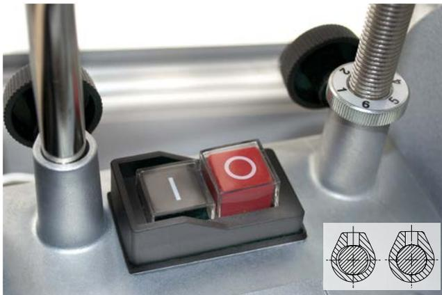
With the sleeves for the Universal Support now being cast in the zinc top, together with the new Tormek stadium shaped design of the holes (patent pending) – the precision have been improved significantly. It will improve your control of the sharpening – and your result.
